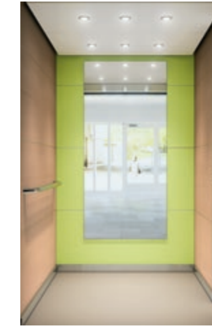
12006 Ceiling: CL88 Cloud White (P50) painted steel, Wall B: Hazel Oak (L202) laminate, Wall C: Lime Green (L207) laminate with mirror, Wall D: Hazel Oak (L202) laminate, Floor: Grainy Sand (SF31) composite stone, Car Operating Panel: KSS D40 Snow White; Aluminum frame with mirror polished finish, Handrail: HR64 Asturias Satin (F) brushed stainless steel, Skirting: Asturias Satin (F) stainless steel
