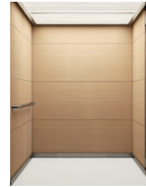
13013 Ceiling: CL151 Asturias Satin (F) brushed stainless steel, Bamboo graphic panel, Wall B: Oak (L219) real wood laminate, Wall C: Oak (L219) real wood laminate, Wall D: Oak (L219) real wood laminate, Floor: Chalk White (SF30) composite stone, Car Operating Panel: KSS 670 Murano Mirror (H) stainless steel faceplate, Handrail: HR64 Murano Mirror (H) polished stainless steel, Skirting: Asturias Satin (F) stainless steel
