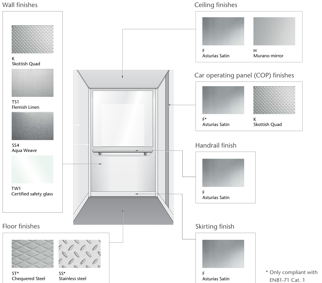
Figure 4. EN81-71 Category 1 and 2 compliant car interior materials
