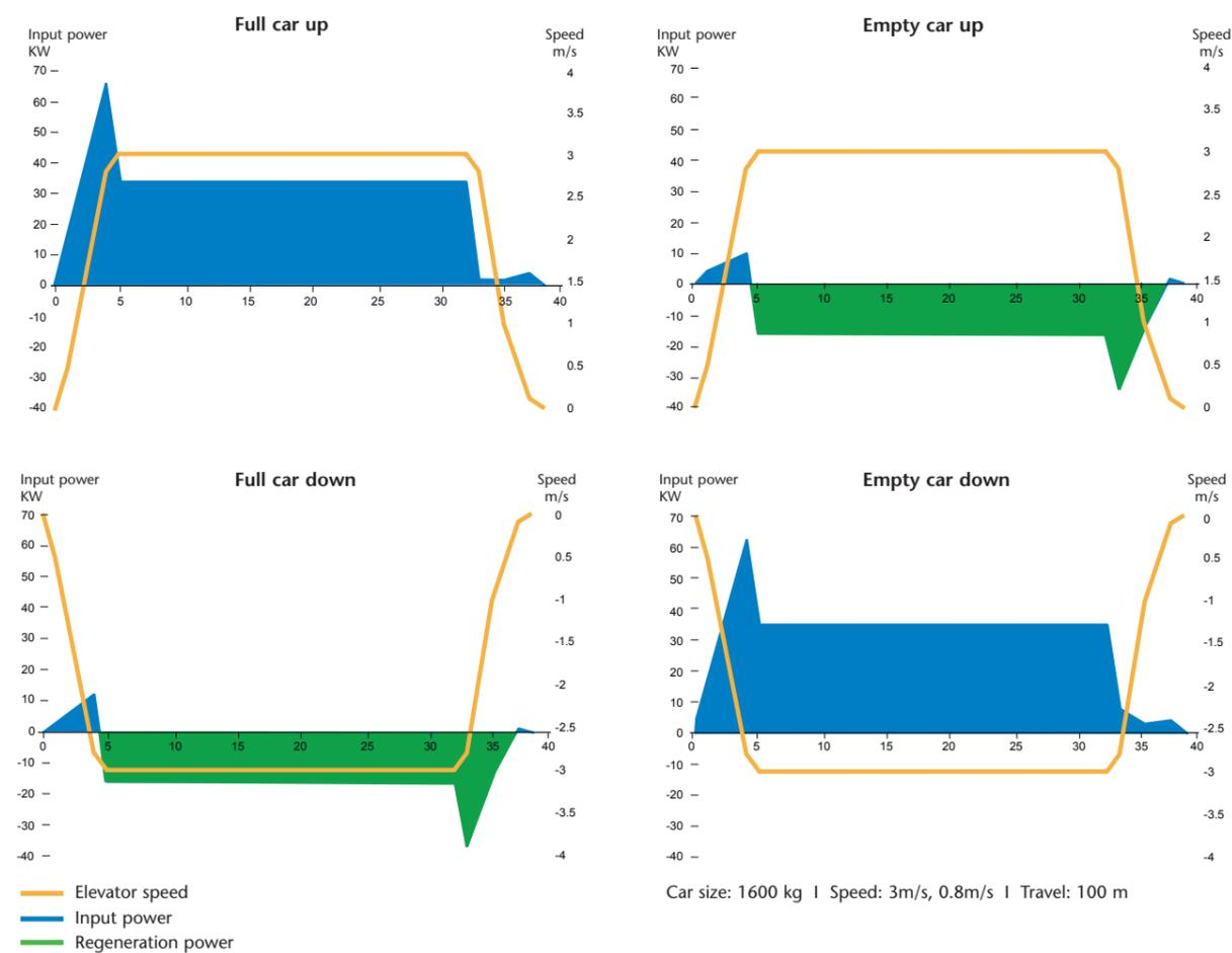
When a full car is going down or an empty car is going up, the system is regenerating energy into the building's power network. So, for most of the elevator's travel time, the system generates energy.
