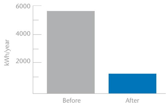
\*Elevator speed 1.0 m/s, load 630 kg, 150,000 starts/year, travel height of 12m and 5 floors.
