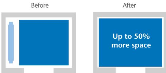
The KONE NanoSpace uses ultra-compact balancing weights, leaving more space for a larger car with no changes to the shaft.
